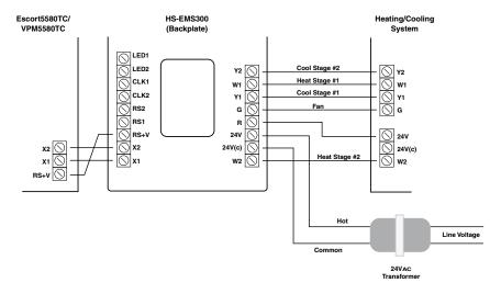
Warning! Remove the internal jumper (shunt) before connecting the stand-alone transformer.
